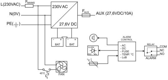
Fig.1. The block diagram of the PSU.
